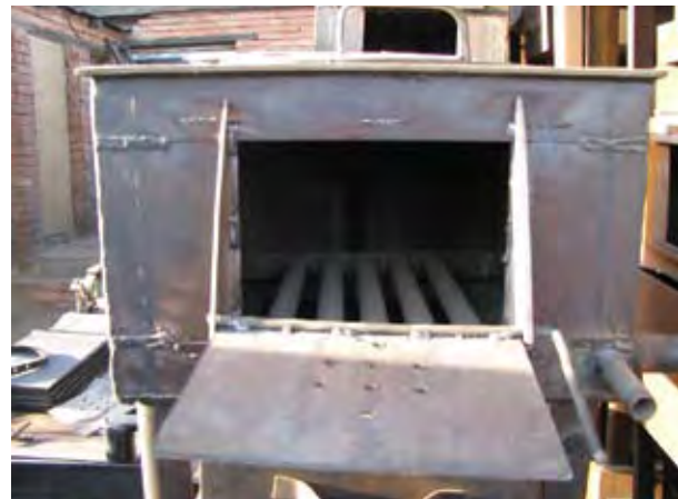
Low-Pressure Boiler Showing Water Pipes
